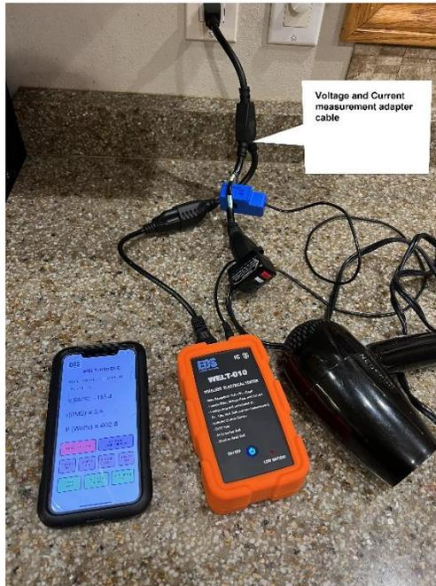
Figure 3 Voltage, Current and Power Measurement
