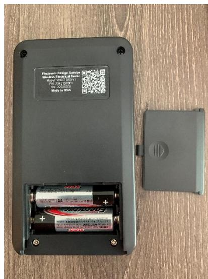
Figure 7 Battery Installation and Serial Number Location
