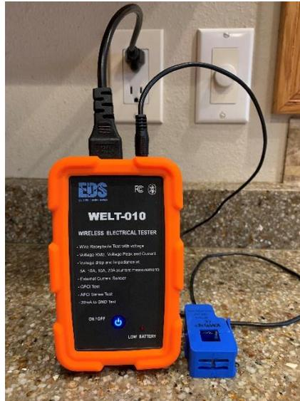
Figure 2 Voltage, Voltage Drop measurements, Socket Monitor, GFCI and AFCI Tests
